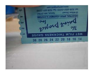
C) Remove the gauge and inspect where paint touched teeth. This is your wet thickness...here seen as 26 mils (or .026").
