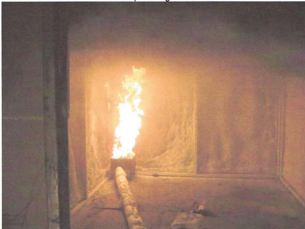
160kW and smoke ceiling
