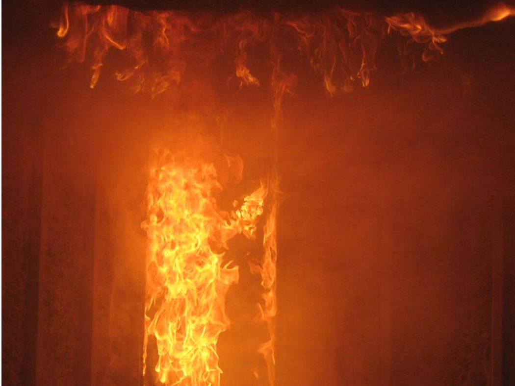
160kW and ignition of ceiling
