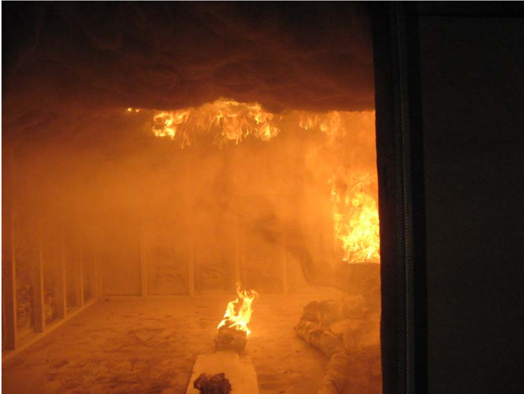
Test photo. Flashover and ignition of paper target.
